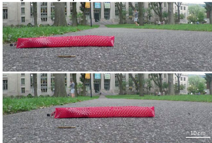
Fig. 5 | Encoding physical intelligence in soft robot bodies. a | Mechanical instabilities can be used to create digital logic gates for binary mechanical computation and human interaction 182 . b | Introducing cuts (kirigami) allows the buckling-induced transformation of flat sheets into 3D textured surfaces, the directional frictional properties of which can enable efficient crawling gaits 187 . c | Strategically developing unequal strains, through a difference of materials 86 in adjacent layers of a composite structure, can achieve programmable deformations and shape morphing. Panel a adapted with permission from REF. 182 , National Academy of Sciences. Panel b adapted with permission from REF. 187 , AAAS. Panel c adapted with permission from REF. 86 , AAAS.
